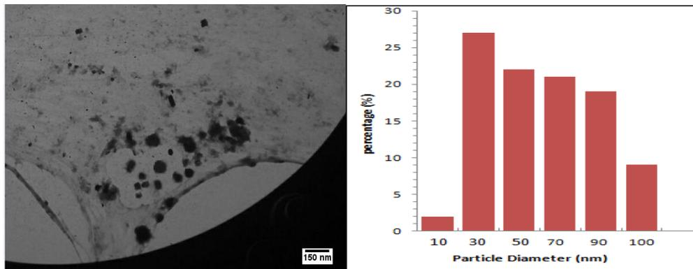
**Fig. 3:** The morphology and particles size distribution of CuO NPs with 500 pulse at  $280\text{nm}$ , 1Hz and  $1064\text{ nm}$ .
