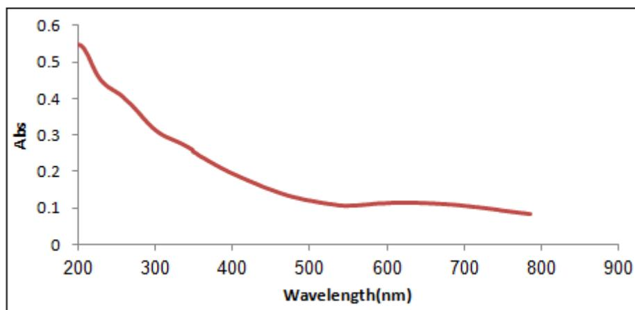
**Fig. 2:** The absorption spectra of CuO NPs at 200 pulse, repetition rate=1 Hz,  $\lambda=1064\text{nm}$  and  $25\text{ mJ/cm}^2$ .
